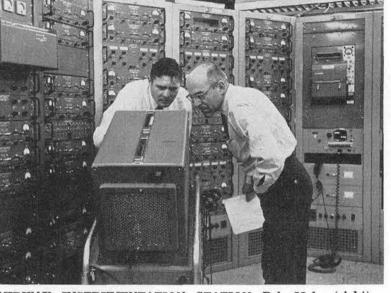
MIDWAY INSTRUMENTATION STATION—Bob Male (right) and Al Britt, chief of FM/FM telemetry unit, monitor wave forms on an oscilloscope just before a Sandia rocket sled firing.
